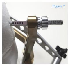
reading is taken at the distal end of the bushing: the full lines immediately to the left of each number correspond to that length of fixation screw and the half lines between them designate intermediate values (Leksell screws are
