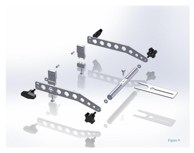
The diagram above may be used as a guide for assembly of the alignment frame components in the event repair or extensive cleaning is required.
