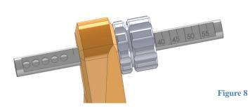
available in increments of 2.5 mm). In Figure 8, the guide scale indicates a fixation screw length of 40 mm at this position. Record the values at each of the sites prior to injection.
